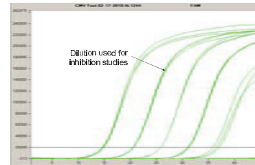
Figure 3: 5 equally spaced CMV amplicon calibrators spanning the linear range of CMV Quantitation from 2x10 7 to 2x10 1 copies per reaction
