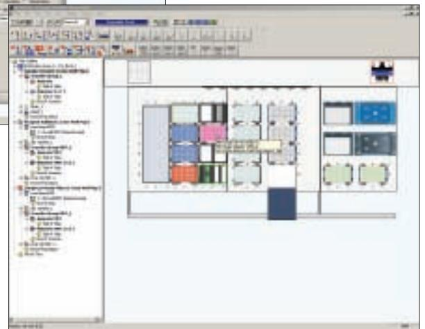
Select the labware on your deck, then drag and drop it onto the pipetting operation step in the test outline where it is to be used.
