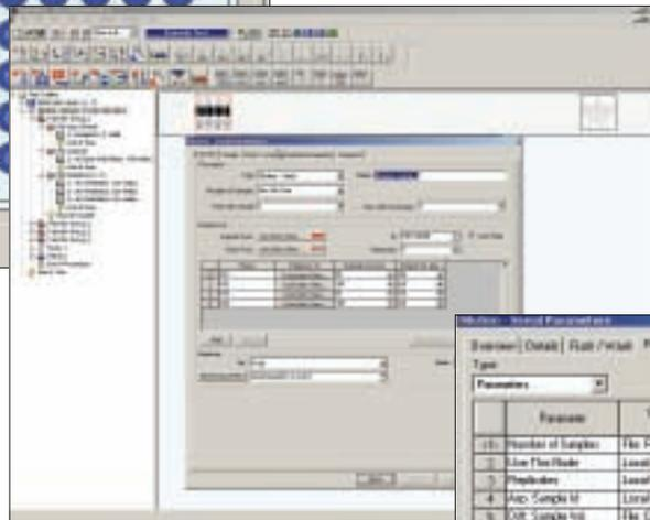
Flexible dilution templates enable easy definition of direct, serial or custom dilution schemes.
