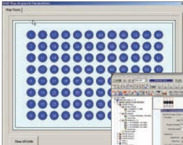
WinPREP's Map Rooms provides flexible pipetting patterns or processing order to be defined or optimized easily.
