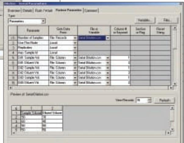
File-based protocols for cherry picking or dilutions can be easily imported into WinPREP. Sample positions or volumes can vary for each sample and be easily imported via Excel® or standard CSV file formats.
